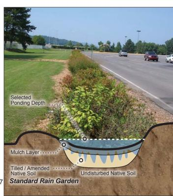
**Standard Rain Garden:** A standard rain garden uses a uniform ponding depth (3" or 6") of water across the entire base of the rain garden. Native soils are used and can be amended if necessary based on the infiltration rate found by the infiltration test. In these systems, the bottom of the rain garden area is raked level with no variation in elevation within the rain garden footprint.
